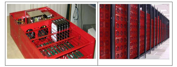
Start with an inexpensive storage appliance rack. The one pictured above left has 3 rows of 15 hard drives, or a total of 45 hard drives. Suppose it were filled out with a Western Digital 10 TB (terabyte) hard drive (say WD Red 10TB NAS) drive that costs \$315 each. The cost to fill the appliance would be \$14,175 for 450 TB (terabytes) of storage.
